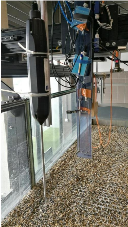
*Head rod and ADV on automated mount in the tilting flume*
