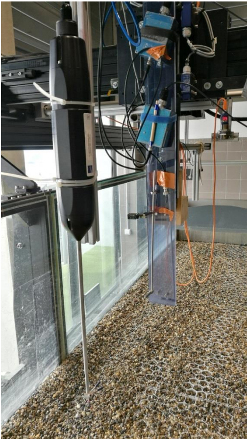
Head rod and ADV on automated mount in the tilting flume
