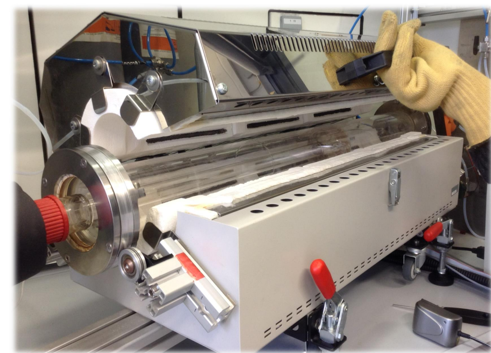
Figure 1. Photo of the Advanced Gas-Ash Reactor showing the working tube within a three-stage furnace
