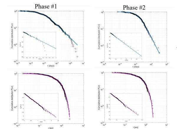
The analysis (figures to the left) indicates that the observed scaling behavior of the waiting times and jump lengths for the two phases of the 2013 earthquake swarm can be well approximated with the q-exponential distribution, exhibiting asymptotic power-law behavior with exponents that correspond to the sub-diffusive regime of the CTRW model.
