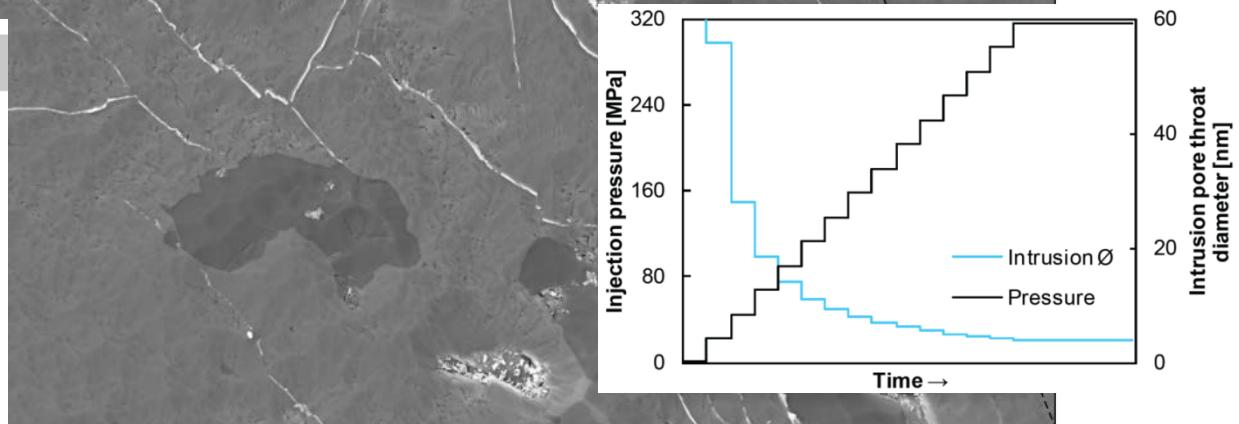
*Wood's metal (in white) injection into cracks*
