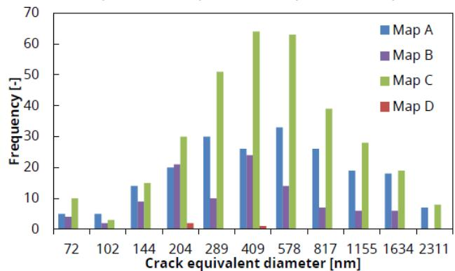
*Equivalent diameter distribution (in nm) for cracks and pores*
