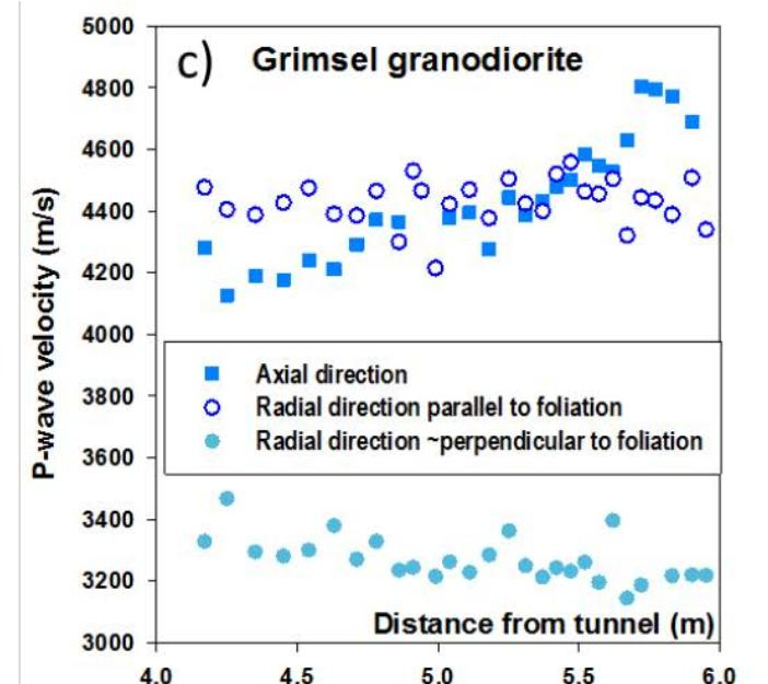
Figure 1. a) Cutting the core into small blocks; b) Measuring the P-wave velocity for quality check; c) P-wave velocity measurements in three orthogonal directions vs. distance from the tunnel.
