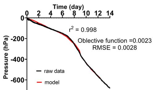
Fig 5: Plot of inversely modelled hydraulic conditions in the column
