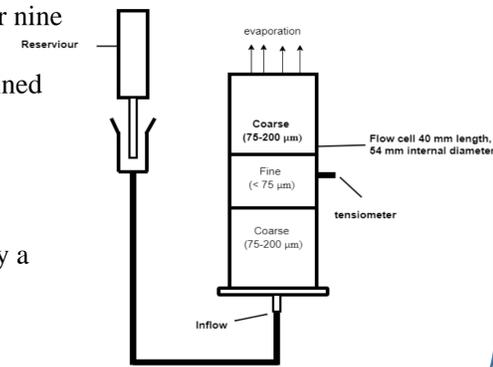
Fig 1: Evaporation Experiment
