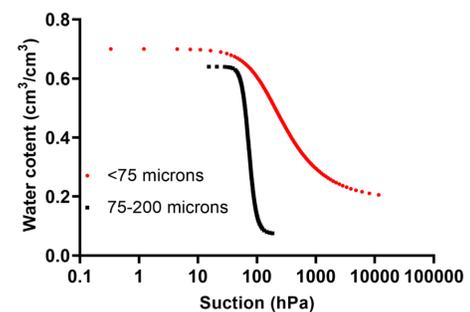
Fig 4: Initial water retention curve for different particle sizes
