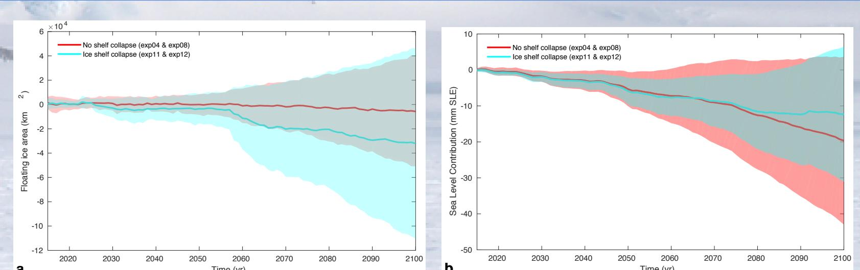
Total Antarctic ice shelf area simulated (a, in km<sup>2</sup>) and sea level contribution (b, in mm SLE) with (b) and without (red) ice shelf collapse over the 2015-2100 period. All results are based on the CCSM4 RCP 8.5 scenario and relative to *ctrl\_proj*.
