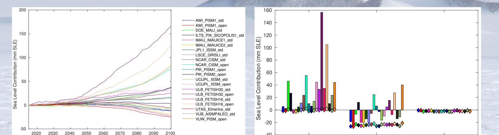
Projected sea level contribution (left, mm SLE) with NORESM1-M RCP 8.5 scenario relative to *ctrl\_proj*. Regional sea level contribution over the 2015-2100 period (right, mm SLE) relative to *ctrl\_proj*. Diamonds represent the additional surface mass balance applied during the 2015-2100 period relative to *ctrl\_proj*.
