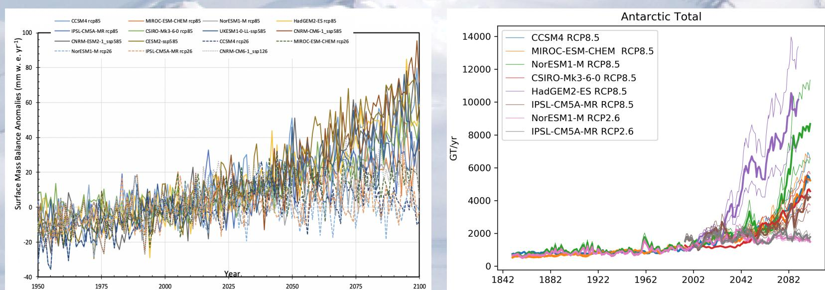
Surface mass balance anomalies (left, in mm w.e./yr) and basal melt (right, in Gt/yr) forcings from CMIP5 AOGCMs. Forcings assume fixed ice sheet and ice shelves geometry
