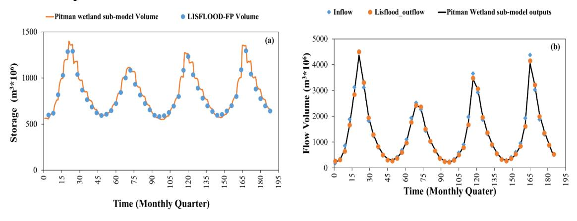
Graphical visualisation of the correspondence of the LISFLOOD-FP and PITMAN wetland sub-model wetland storages at Ankoro wetland system based on 270 m model resolution. (a) the Pitman wetland sub-model reproduced well the wetland storages and (b) the Pitman wetland sub-model was able to reproduce the outflow.
