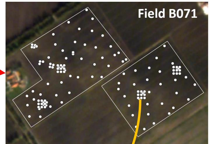
Current sampling according to a  $30 \times 30$  m Elementary Sampling Unit with 10 points
