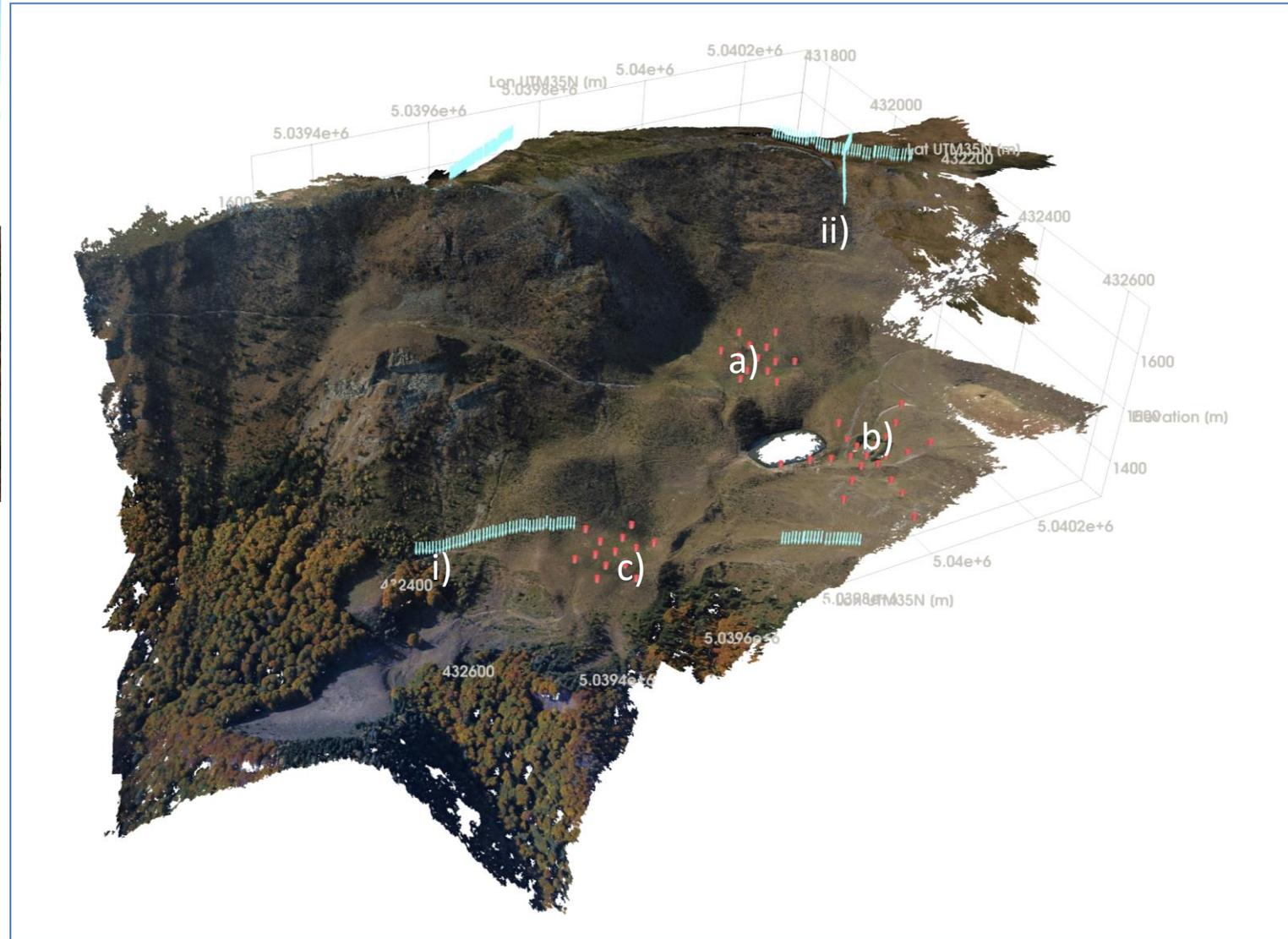
UAS based landscape photogrammetry: red cylinders indicate the installed seismic networks and the light blue arrows represent the performed SRT profiles
