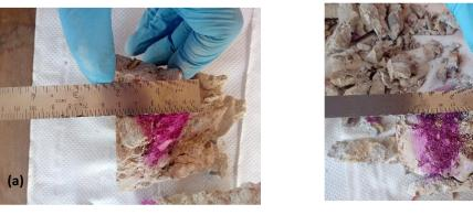
Results of the phenolphthalein indicator test for D3 (a) and D4 (b) concrete samples.
