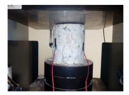
Test layout used in the uniaxial compression Image of the D3 sample at failure in compression test of the concrete core-drillings.
