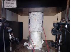
Test layout used for the estimation of the elastic modulus of concrete core-drillings through the application of strain gauges
