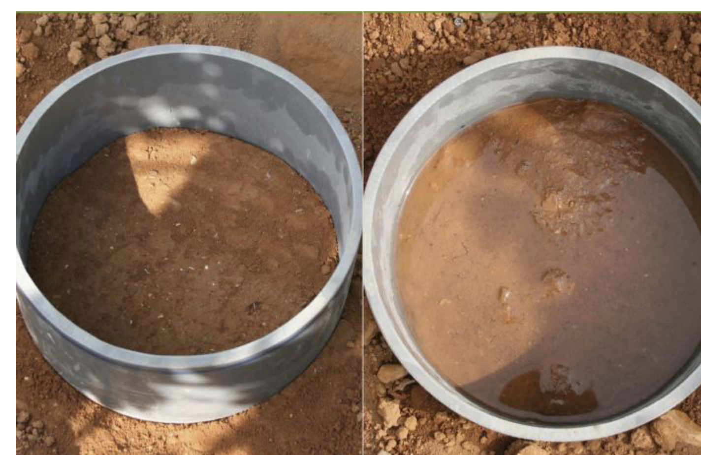
Fig. 1 Single ring infiltrometer
