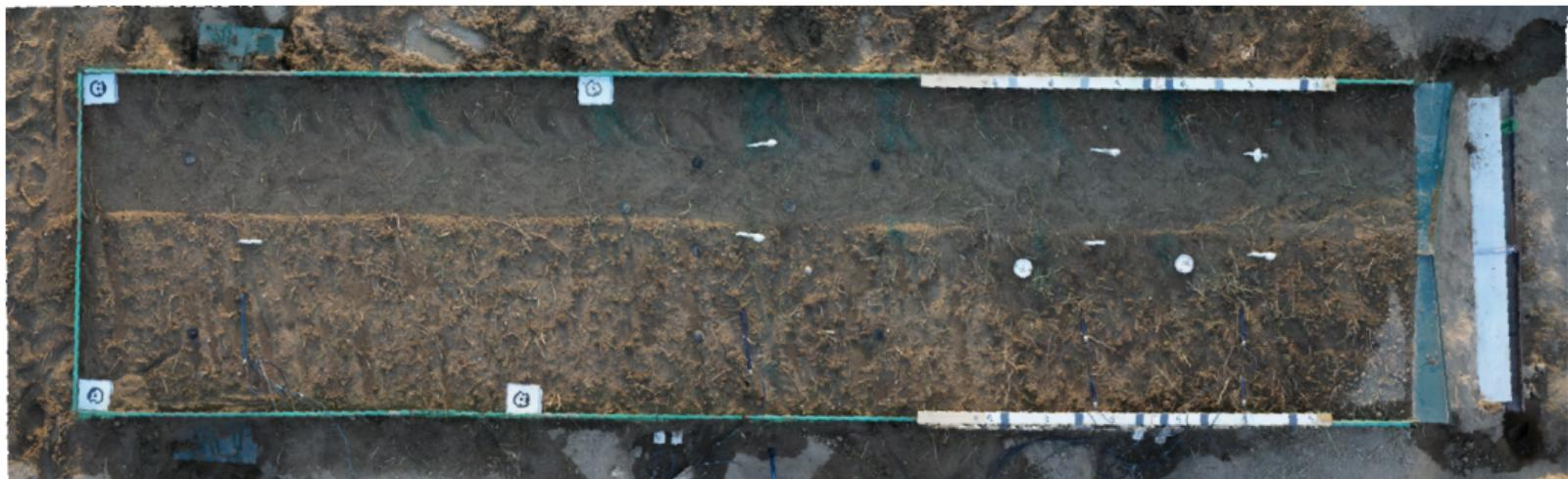
Surface roughness was calculated for each of the experimental plots based on the before and after rainfall surface conditions.
