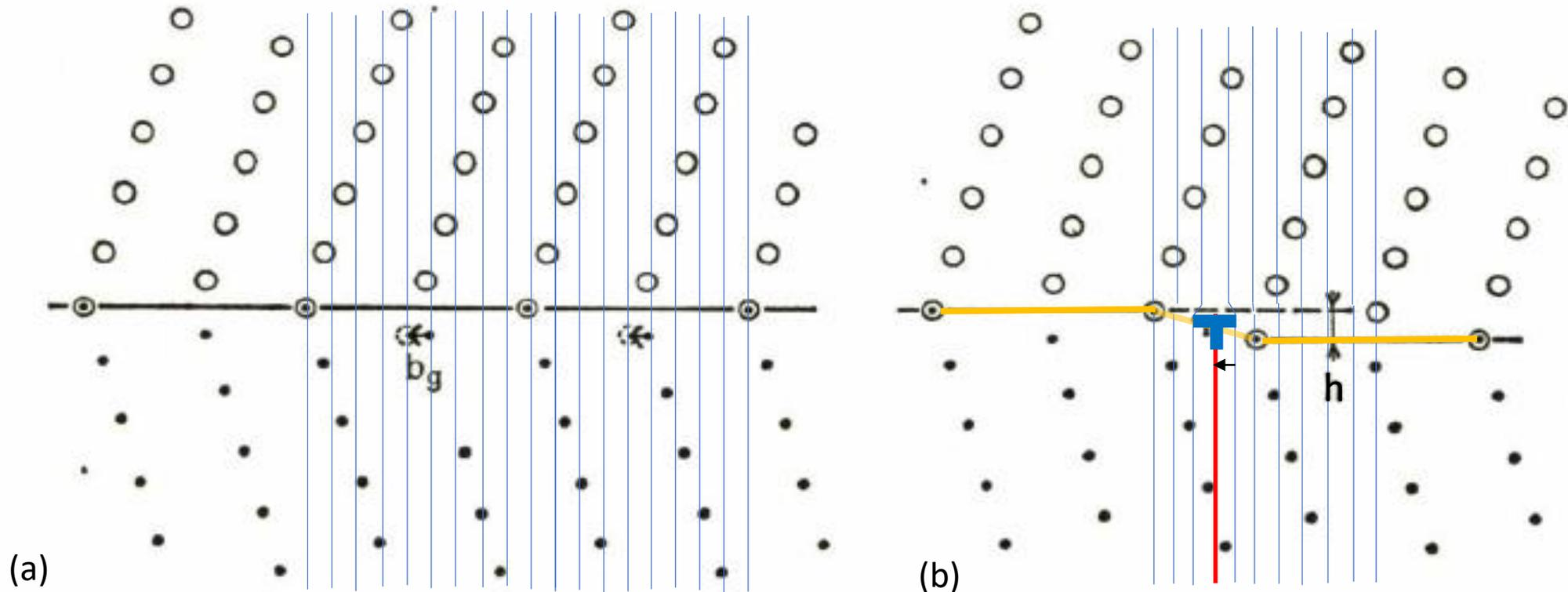
The shear displacement observed in ice (Figure 4) fits with the disconnection model<sup>13,14</sup>. (a) CSL model for a 34° tilt boundary in ice. The blue lines are part of the DSC which defines the Burgers vectors of grain boundary dislocations<sup>8c</sup>. (b) A shift of the lower left part of the black lattice by  $b_g$ , produces a disconnection. The extra half plane of the dislocation is shown in red. Motion of the disconnection produces shear and GBM.
