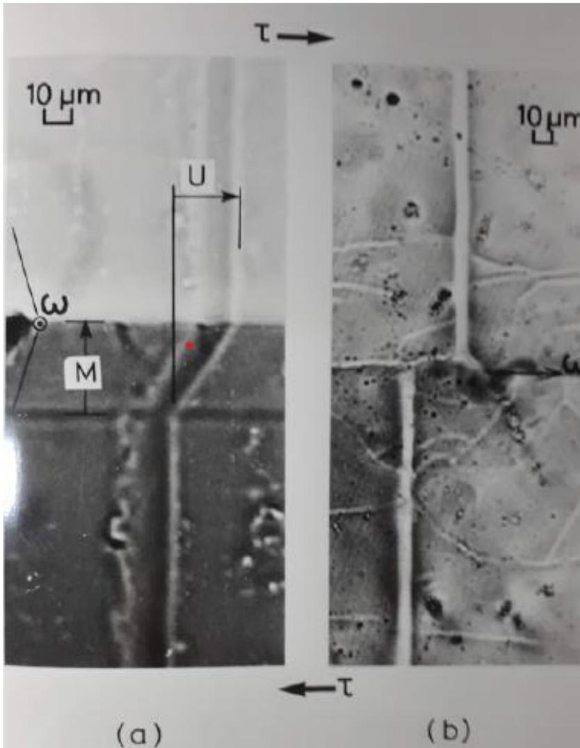
Two examples of grain boundary displacement in experimentally deformed ice bicrystals, at conditions similar to that found in natural ice.
