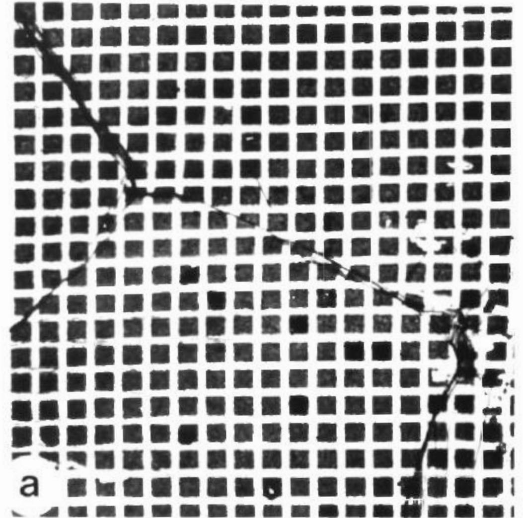
Deformation at grain boundaries revealed from displacements and distortion of marker grid<sup>12</sup>.
