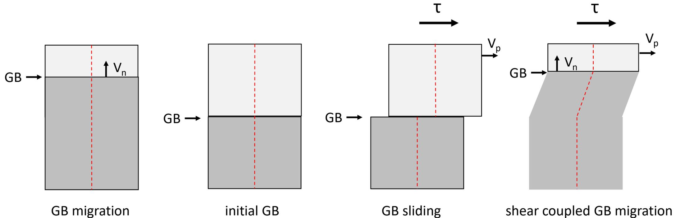
Diagrams illustrating different types of GB behavior:  $V_n$  = velocity of migration,  $V_p$  = velocity of translation parallel to boundary. Conventional view of GB migration as recovery processes. Under shear stress,  $\tau$ , deformation can occur by GB sliding or shear coupled migration.
