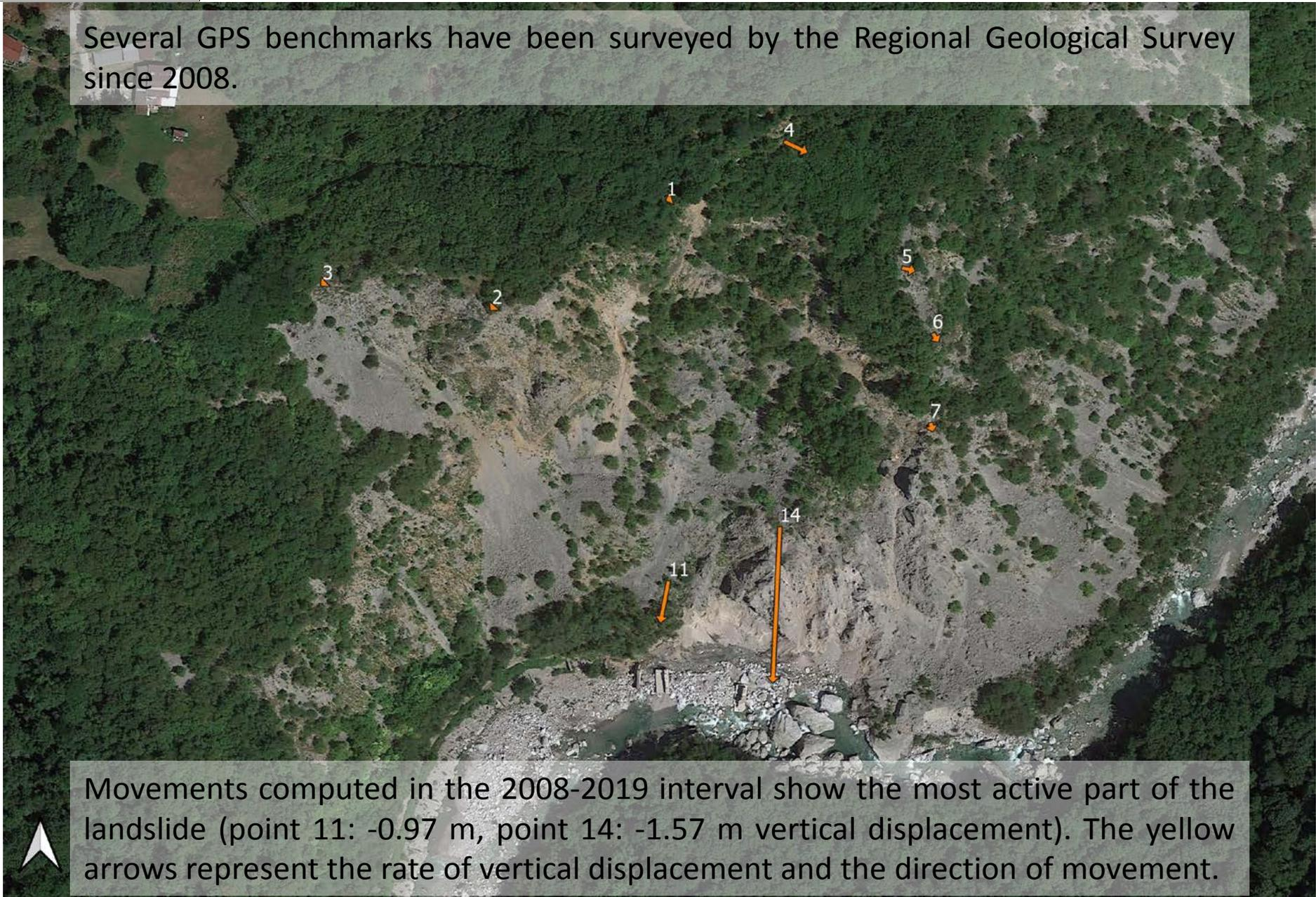
Movements computed in the 2008-2019 interval show the most active part of the landslide (point 11: -0.97 m, point 14: -1.57 m vertical displacement). The yellow arrows represent the rate of vertical displacement and the direction of movement.
