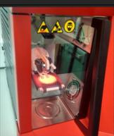
Glass beads analyses, using a X-ray Fluorescence S2-PUMA
