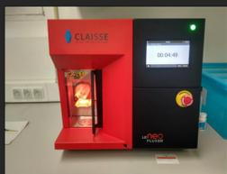
Glass beads preparation, using 12g flux + 1,2g sample
