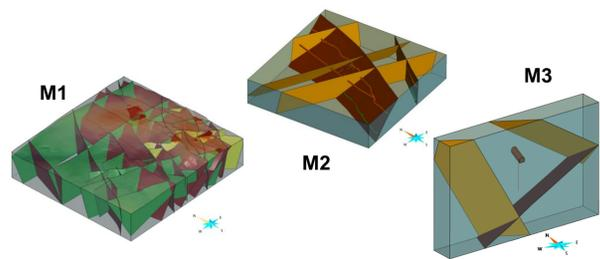
Fig. 1: a) Large scale model M1 (2500x2500x500 m) with 43 faults and mine drifts. Used to calculate stress tensors at small scale model boundary. b) Small scale model M2 (250x250x50 m) with 5 faults and mine drifts used to calculate in situ stress field at the investigation site. c) Slice model M3 (70x10x50 m) with 3 faults and mine drift used to investigate the influence of a potential EDZ around the drift. The test site is centred in the large and small scale models.
