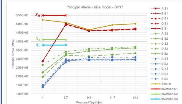
Fig. 7: Resulting principal stresses for BH17 from model M3. Horizontal principal stresses do not differ much between scenarios. Stress regime is strike slip for M3. Solid lines represent TF stressfield magnitudes from Inversion results.
