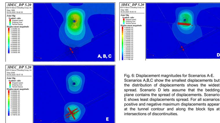
Fig. 6: Displacement magnitudes for Scenarios A-E. Scenarios A,B,C show the smallest displacements but the distribution of displacements shows the widest spread. Scenario D lets assume that the bedding plane contains the spread of displacements. Scenario E shows least displacements spread. For all scenarios positive and negative maximum displacements appear at the tunnel contour and along the block tips at intersections of discontinuities.
