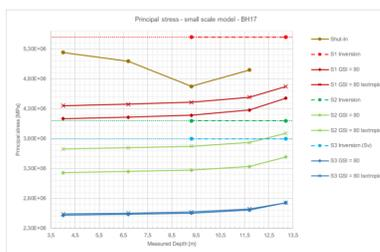
Fig. 4: Results for M2 in BH17. Inversion results of the measurements show a thrust faulting stress regime and strong increase of magnitude for horizontal principal stresses (1-2 MPa). Vertical stresses from inversion data and isotropic M2 correspond well (S3 Inversion - cyan, S2 Isotropic - green). However, M2 delivers a strike-slip regime for BH17.
