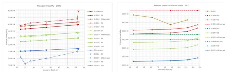
Fig. 3: Results for M2 in BH10. Principal stresses for different GSI-values and corresponding boundary stress fields from M1. Inversion data from project partners at RUB for BH10 measurements were used for validation. For better comparison with the inversion data, we calculated one model with isotropic elastic constitutive law.
