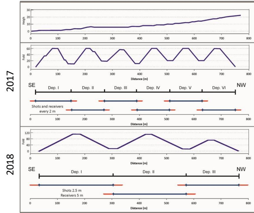
Schematic acquisition geometry
