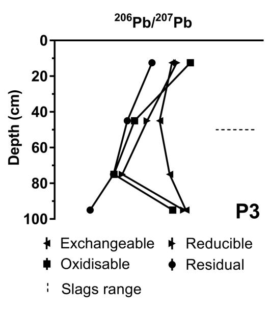
Step 3 – oxidizable (organic matter and sulphides), H<sub>2</sub>O<sub>2</sub> (85 °C) then 1 mol I<sup>-1</sup> CH<sub>3</sub>COONH<sub>4</sub>.
