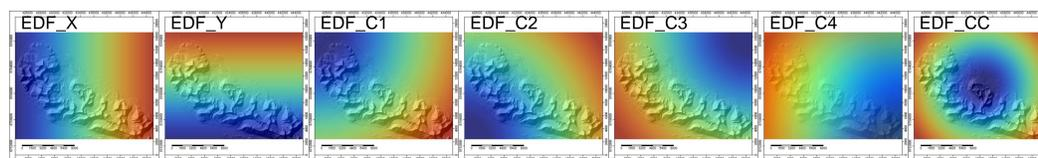
Fig. 3: Euclidean distance fields (EDF) representing the Euclidean distance to the left (EDF\_X) and bottom boundary (EDF\_Y), upper left (EDF\_C1), lower left (EDF\_C2), upper right (EDF\_C3) and lower right corner (EDF\_C4) and the center (EDF\_CC) of the study area.
