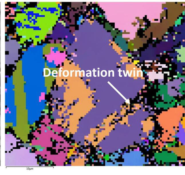
Granulite sample deformed at 2.5 GPa, 850 °C and  $10^{-6}$  s $^{-1}$  in the Griggs apparatus at ENS Paris. Experiment performed by Marie Baisset
