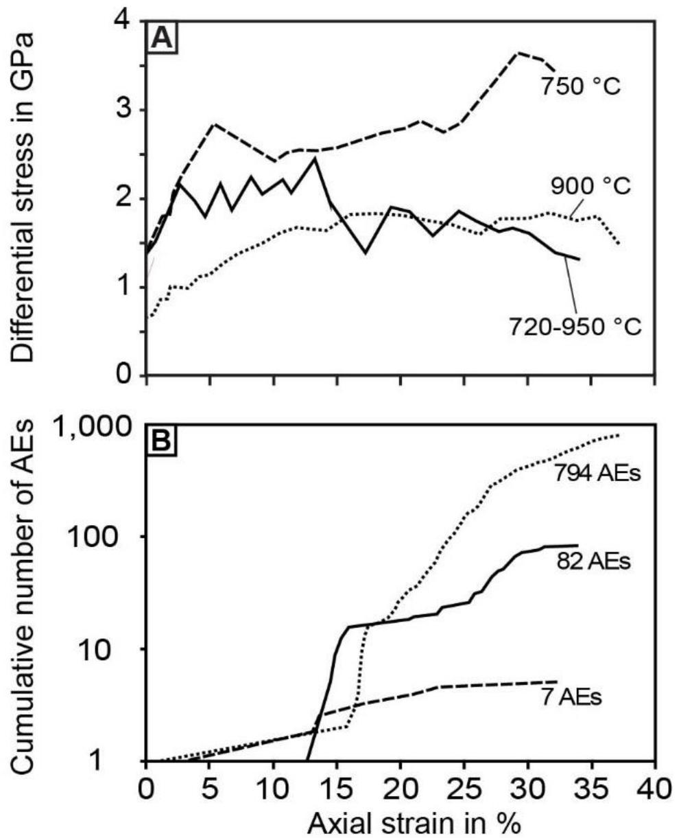
The stress-strain evolution (A) as well as the cumulative number of AEs versus axial strain (B) are shown for the tree experiments that were all performed at 2.5 GPa confining pressure and a strain rate of  $5 \times 10^{-5} \text{ s}^{-1}$  but at different temperatures.
