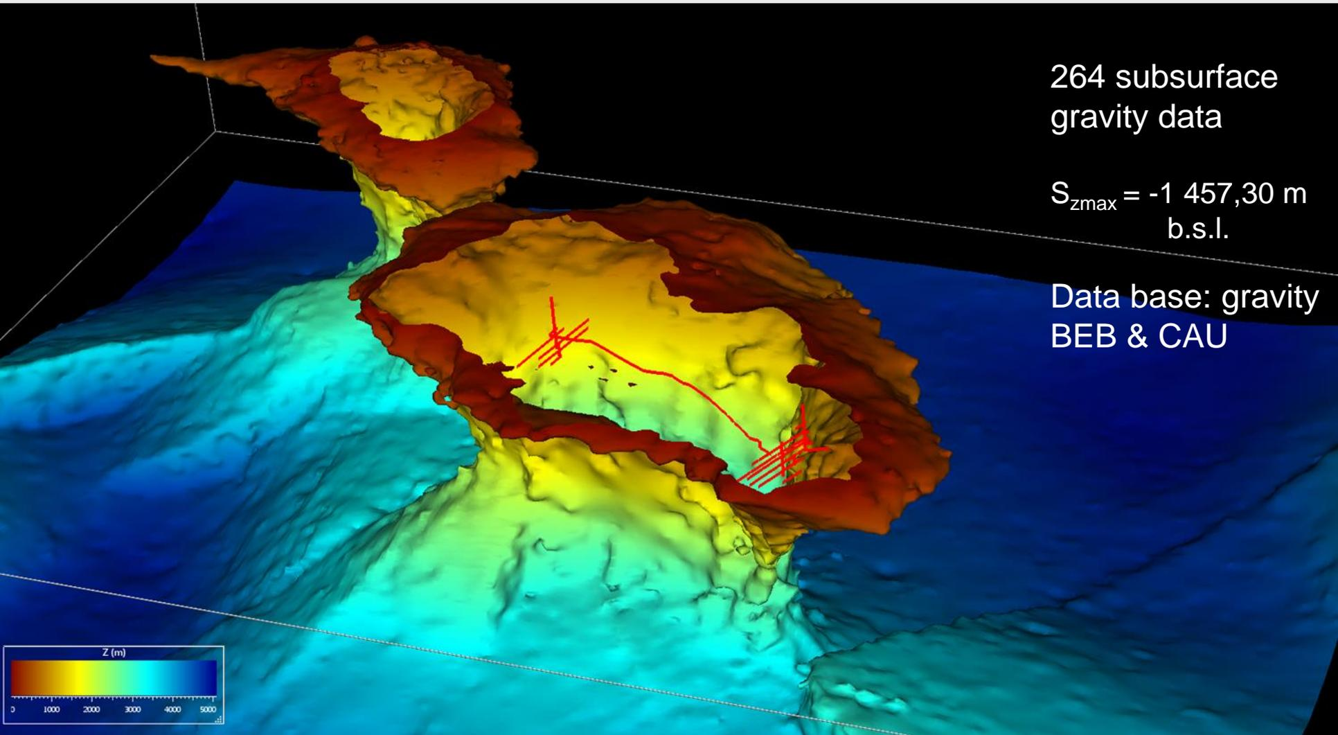
The task: How to verify / test a salt structure provided by a **3D seismic survey** using **existing old gravimetric data** (gravity, torsion balance).
