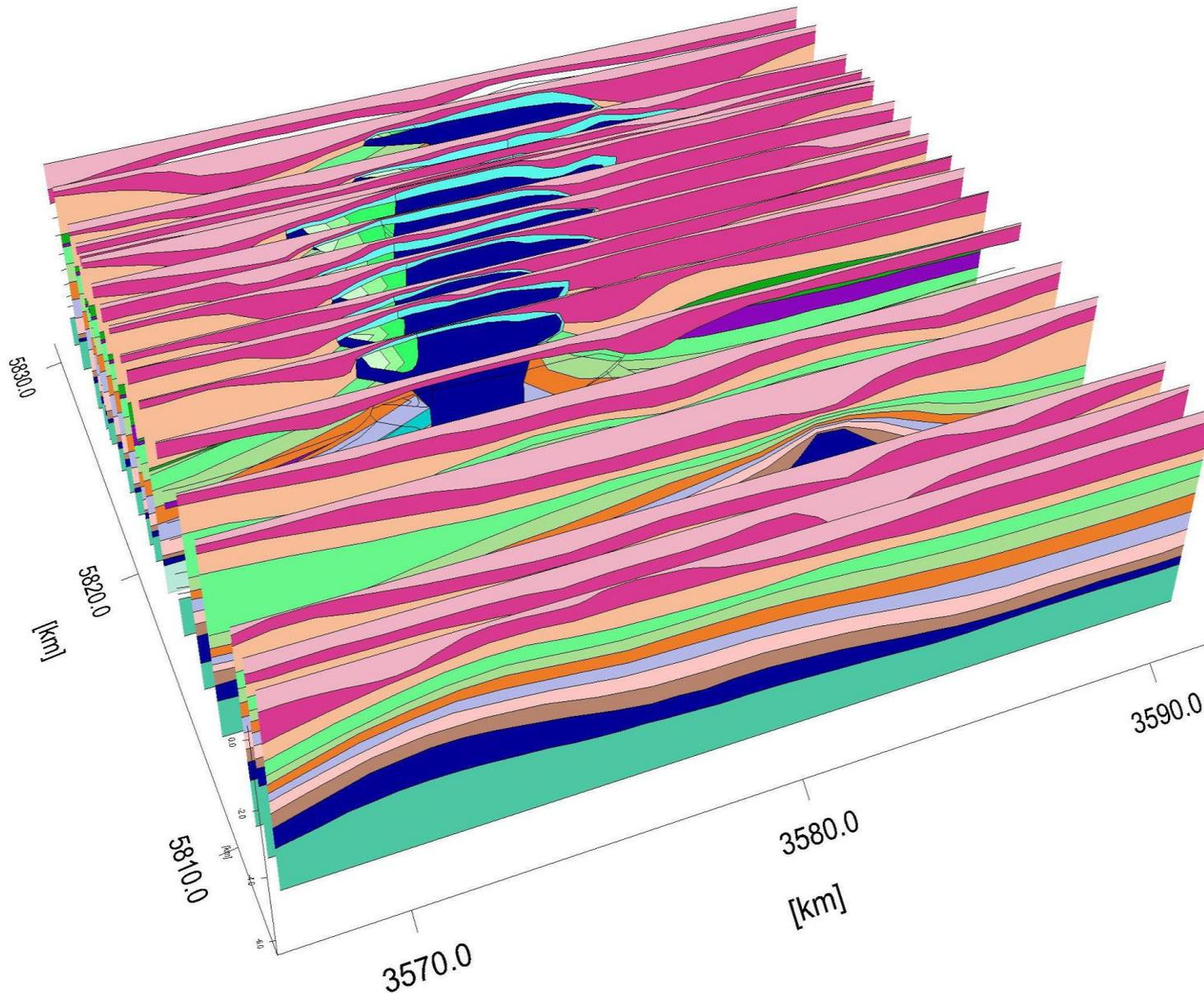
Salt dome is modelled by **17 vertical cross sections** - to define the 3D model structure of a salt dome.
