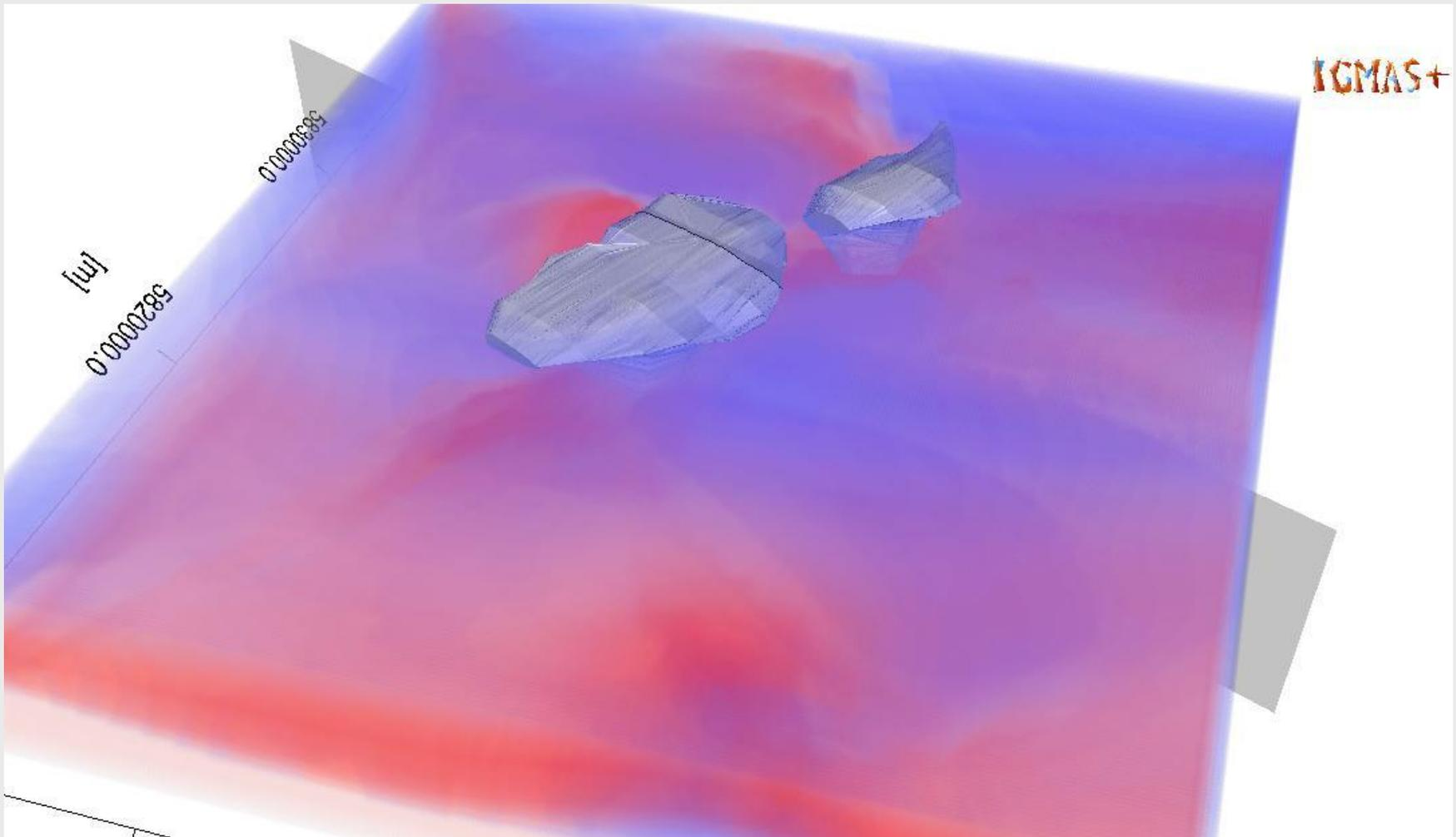
The complete 3D velocity model of the Gifhorn Trough – transferred into a 3D voxel density model which surrounds the fixed density polyhedron model of the salt dome.
