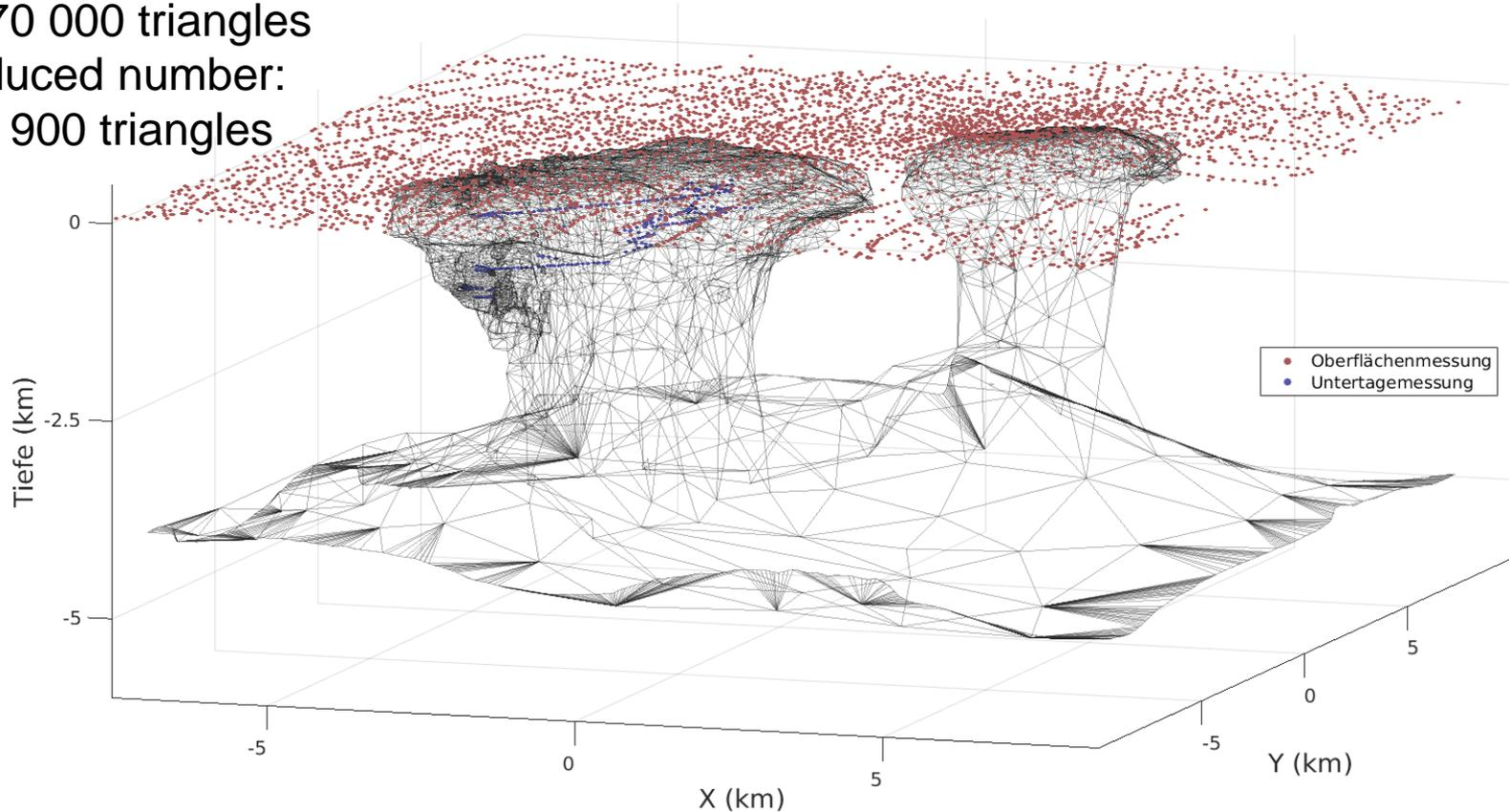
Parameter reduction: here reduction of triangles – without loss of gravity effect which is smaller than 1 % ... (Götze, Schmidt & Menzel, 2017)
