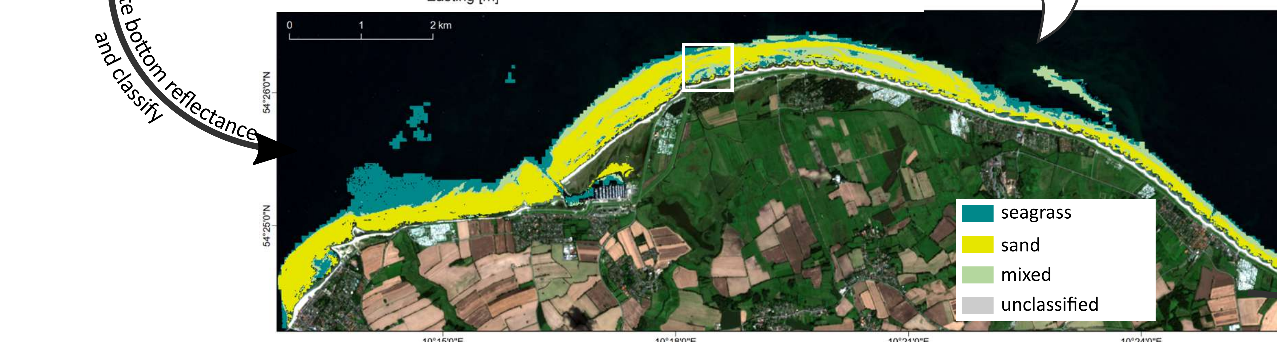
Fig. 3: Classified sea bottom based on Sentinel-2B bottom reflectance (23 Aug 2017). The intermediate steps to retrieve bottom reflectance are not shown here.
