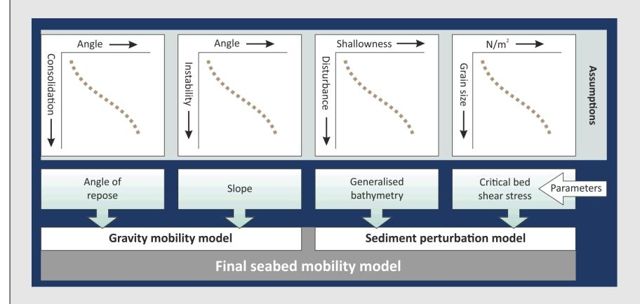
Notes for online sharing: General workflow summarised as: (1) establish and code assumptions based on sediment properties; (2) build initial rasters (which are models themselves) to use as model parameters; (3) sum parameter values to create overall seabed stability probability model.
