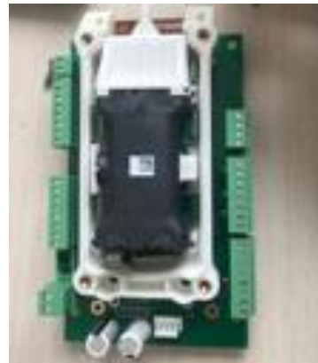
CO 2 Sensor (SenseAir AB HPP_CO 2 3.2version )
