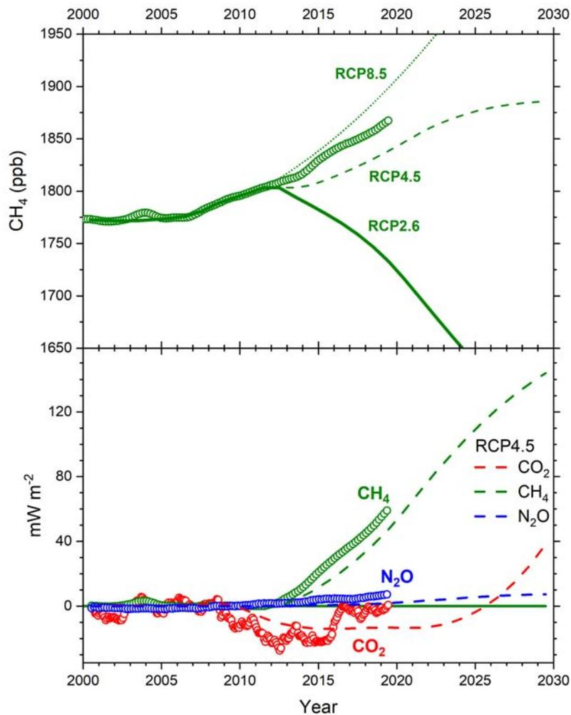
Top: Global methane (green) compared to RCP2.6 consistent with the Paris Agreement and other scenarios. Lower: actual differences in radiative forcing from RCP2.6 methane (green),  $\text{CO}_2$  (red), and nitrous oxide (blue).
