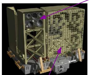
MMIA: 3 photometers (777nm, 337nm, 180-230nm) 2 cameras (optical) Flash images
