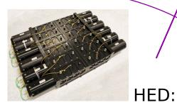
300 keV - 30+ MeV, <1 us 12 BGO Lightcurves Cross-trigger between MMIA and MXGS, <10us relative timing accuracy
