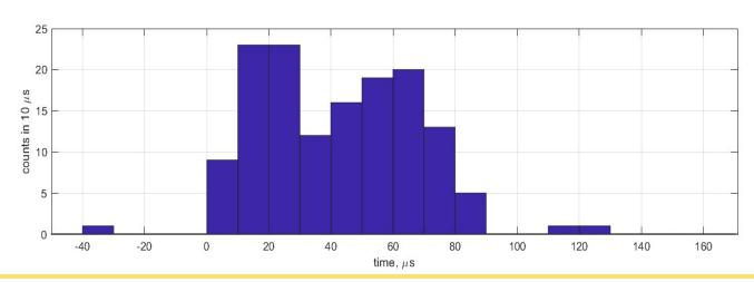
Dip = detector saturation (this is not a multipulse TGF)
