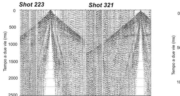
Example of two energizations after ground force correlation. Note on shot 223, the periodic noise induced by the passage of cars at the end of the line (right), which does not, however, mask the strong reflection at TWT at 750 s. Shot 321 records only random noise.
