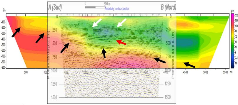
The joint interpretation of DERT and seismic data allowed to reconstruct the 'local' stratigraphic-depositional evolution until a depth of about 1 km, and to highlight the occurrence of a sin-depositional Quaternary tectonic tilting associated to the growth of a fault-propagation fold.
