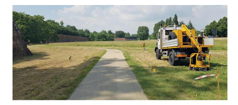
Recently several seismic surveys was performed in urban environment by using frequency-controlled vibroseis sources both in P- and SHwave.
