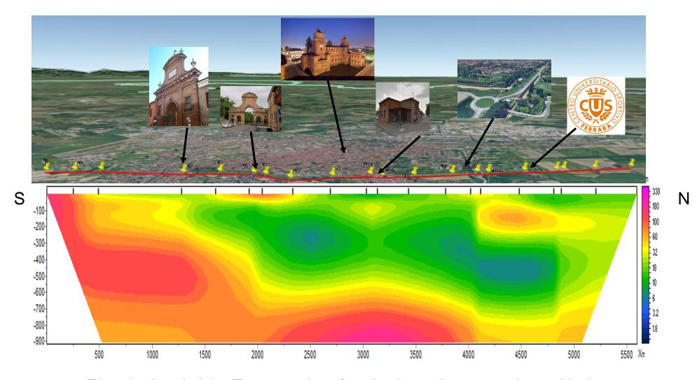
Electrical resistivity Tomography after the inversion procedure with the ZondRes2D software
