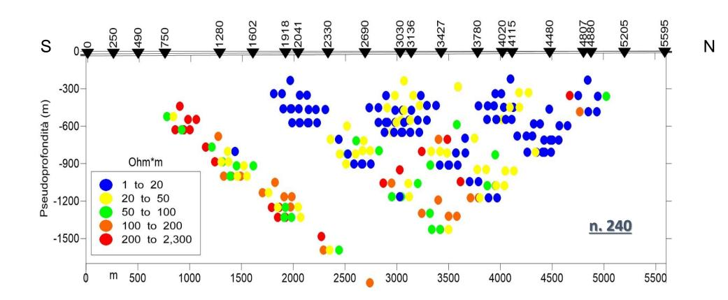
Distribution of the apparent electrical resistivity values obtained from the elaborated acquired data
