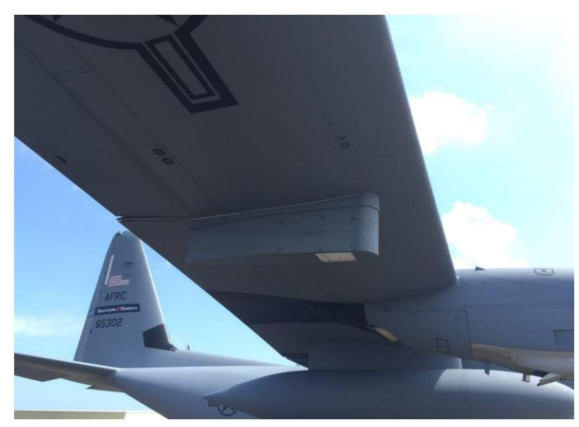
Radiometer under the wing
