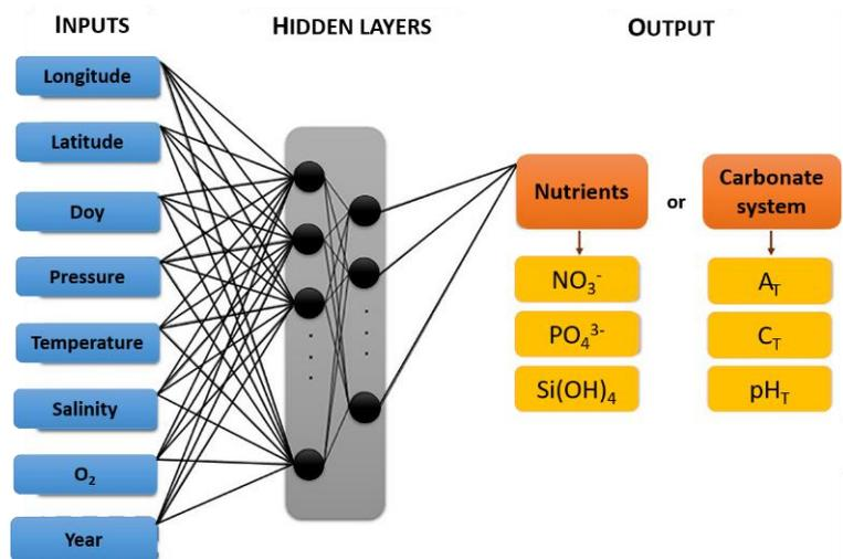
Figure 1: Schematic representation of the architecture of the neural networks, adapted from <sup>4</sup>.
