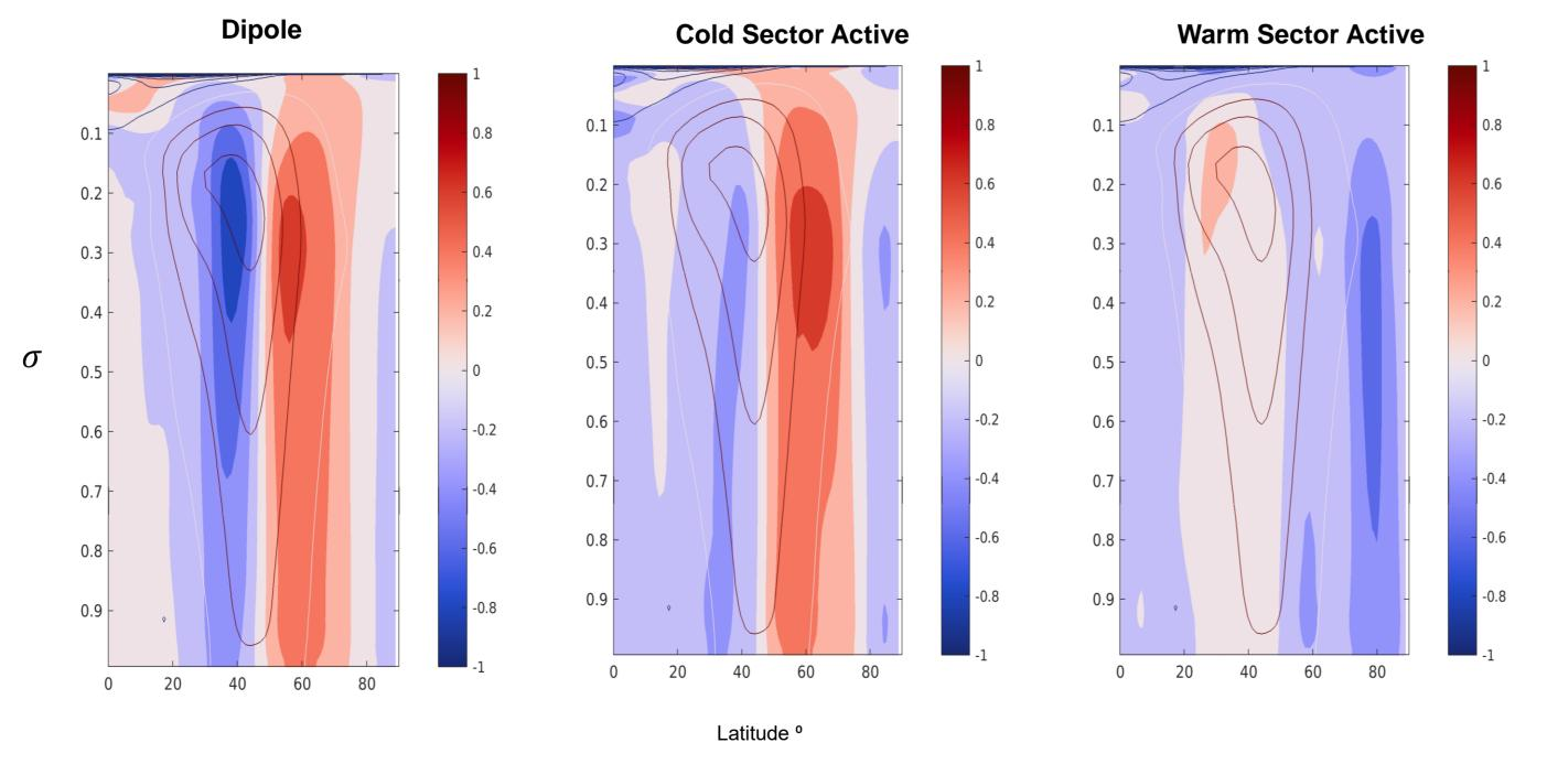
[shadings] Zonal mean zonal wind response (m/s) [contour] Zonal mean zonal wind profile in the control experiment (10 m/s)
