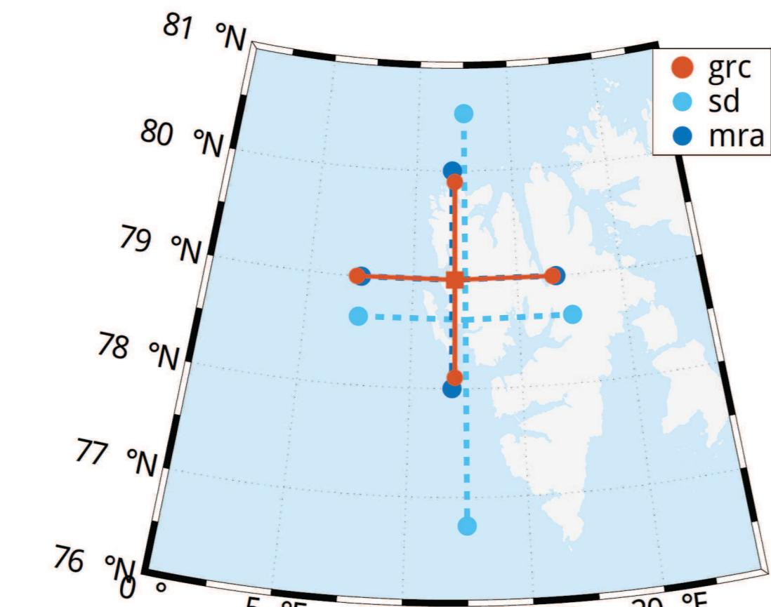
GROMOS-C is state of the art radiometer with beam steering capability covering the four cardinal directions to infer spatial gradients in the ozone volume mixing ratio (VMR) (Schranz et al., 2020). Further, GROMOS-C can be used for horizontal wind observations. The map shows the GROMOS-C beam positions at the stratosphere and the grid points next to these from MERRA2 and WACCM-SD.
