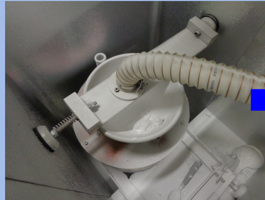
Regolith ice, (5 \mu\text{m} grains, 0.3 g/cm 3 )
