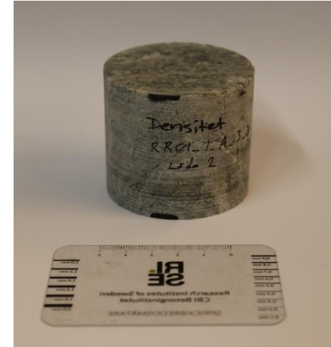
Material for density, porosity, UCP
