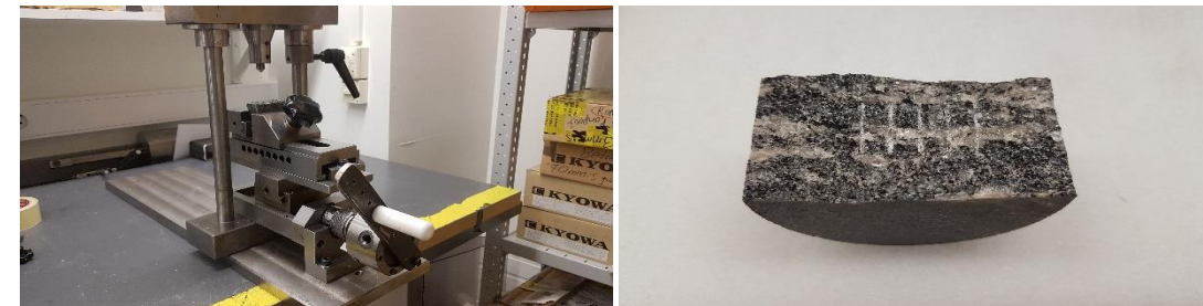
Test of abrasiveness (Cerchar Abrasiveness Index)
