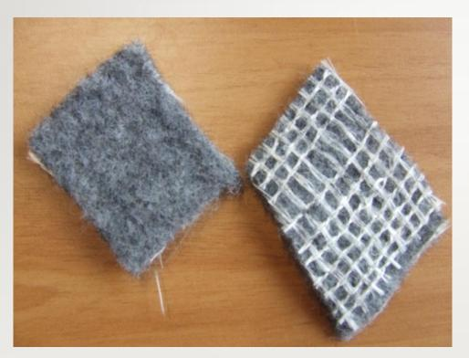
A biodegradable, so-called "green" geotextile was proposed and laboratory tests done.
