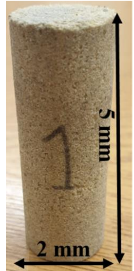
Image of one of the synthetic sandstone used in this study (Rice-Birchall et al., 2021) submitted IJRMMS
