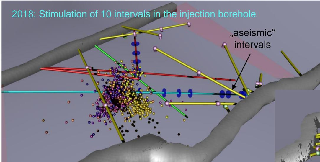
Same injection scheme in all intervals, markedly different seismic response
