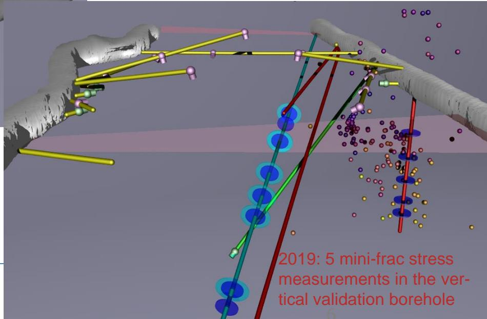
2019: 5 mini-frac stress measurements in the vertical validation borehole
