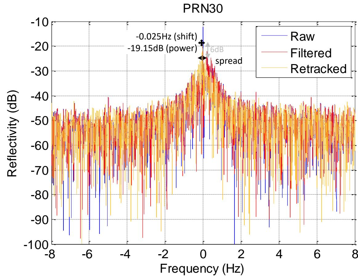
Sharper, higher Power Spectral Density, with lower shift: indicative of a calmer sea
