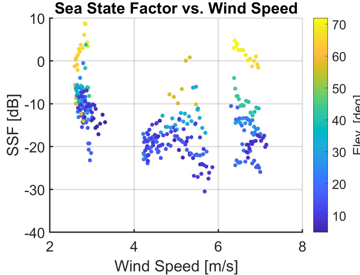
At similar elevations, the Sea State Factor globally increases (in absolute value) with the wind speed.
