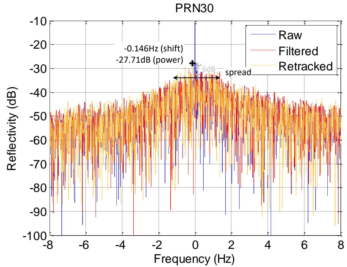
Wider, lower Power Spectral Density, with larger shift: indicative of a rougher sea
