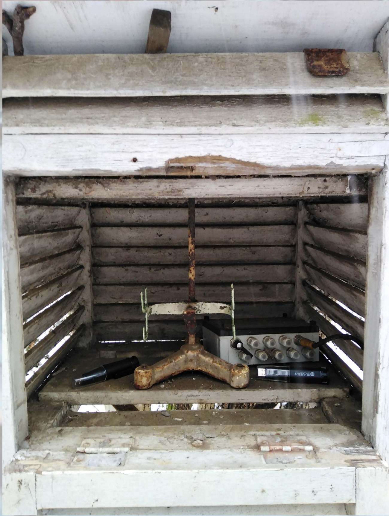
Figure 5: Two portable temperature-RH data loggers in the meteorological station located in Hidegvíz-valley.
