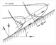
Coupled equations for slope-normal profiles of along-slope wind speed  $(\overline{u})$  and potential temperature  $(\overline{\theta})$
