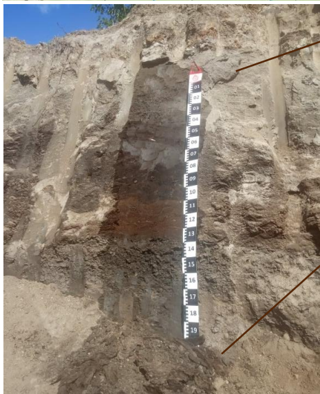
1- Weichselian cover loam, 2- gray medium loam, 3-7 – peat, 8 - dark gray light loam (gyttjia), 9 – gyttjia, 10 - alluvium sand, 11 - fluvioglacial alluvium.
