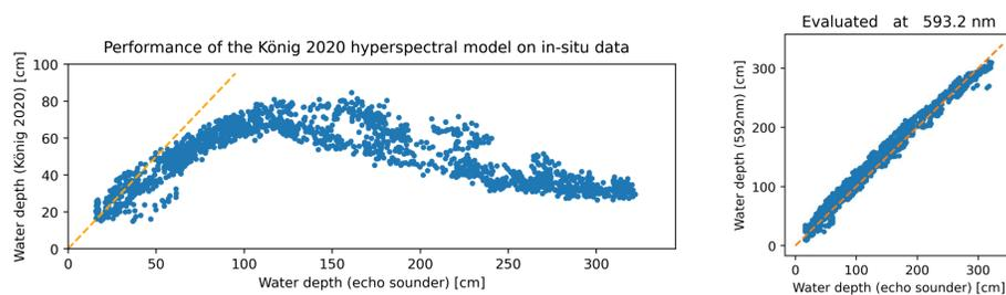
Figure 3. Left panel: König et al. (2020) hyperspectral model vs. echo sounder depth, both measured in-situ by *Böötle* on 9<sup>th</sup> July 2020. Right panel: model re-fitted and evaluated at 593nm instead of the original 710nm, but without the generalization for different solar zenith angles.
