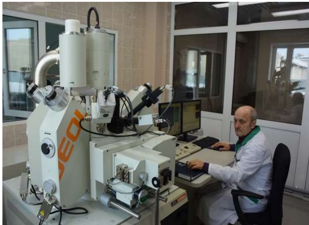
Fig.3. X-ray spectral microanalyzer JXA-8230 in the laboratory of NIGP AK ALROSA systems EX-943100FL1Q, RESO 129eV. Ivanov A. as a microprobe operator.
