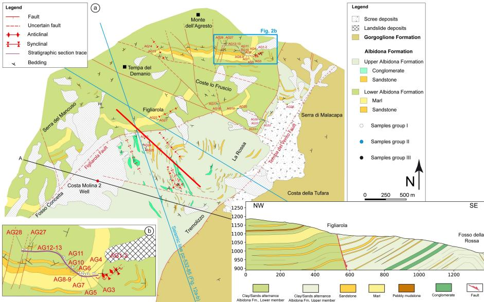
Geological map of the Costa Molina - Monte dell'Agresto-Tempa del Vento area, showing the location of the studied stratigraphic section (b), collected samples and seismic lines. Cross section (c: red line in the geological map) illustrates the relationships between the two members of the Albidona Formation.
