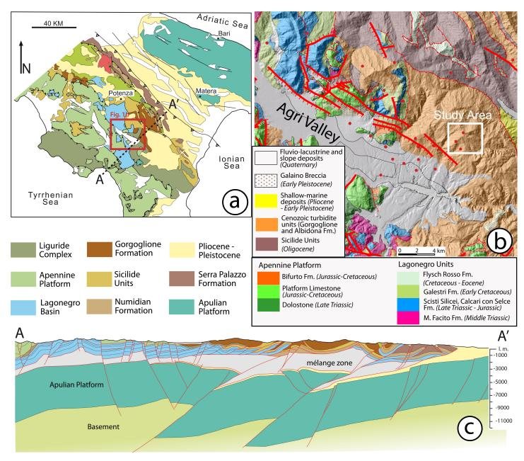
(a) Regional geological map of the Southern Apennines; (b) Sketch map of the Val d'Agri tectonic graben showing the location of the study area. The study area is located in a major outcrop of Miocene turbiditic units. (c) Schematic geological crosssection outlines the structural highs of the Internal Apulian Platform and the geometry of the overlying allochtonous units.
