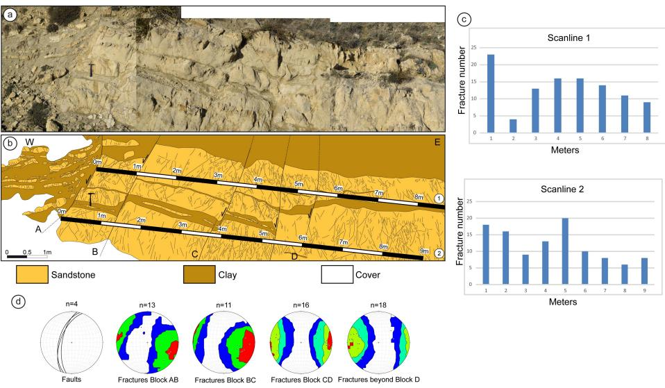
Minor antithetic faults, identified by letters A to D, in the Gorgoglione Formation exposed at the hangingwall of the Figliarola Fault. a) outcrop photograph. b) interpretation showing the position of two scanlines measured along two main sandstone beds. c) diagrams of the fracture intensity measured along the two scanlines. d) stereoplots showing the orientation of fault planes and fractures in each fault-bounded block shown in b).
