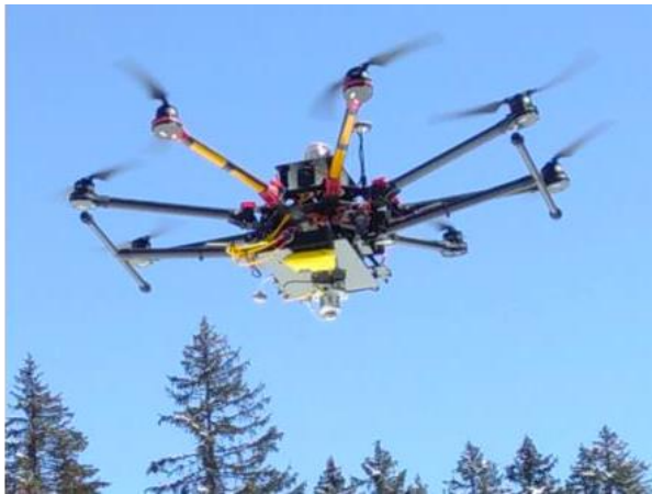
'Albedo drone' with up-and down-looking shortwave radiometers and down-looking hemispherical camera
