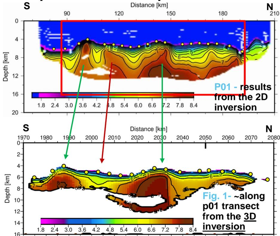
**Figure:** **TOP**) Results of the 2D velocity modelling along P01 using the tomo 3D code (Van Avendonk et al., 2017; Grevemeyer et al., 2019). **BOTTOM**) Results of the 3D inversion at X=425.000 (Fig. 1 in map). Green and red arrows indicates *good* and *bad* correlation of velocity anomalies between the two models.
