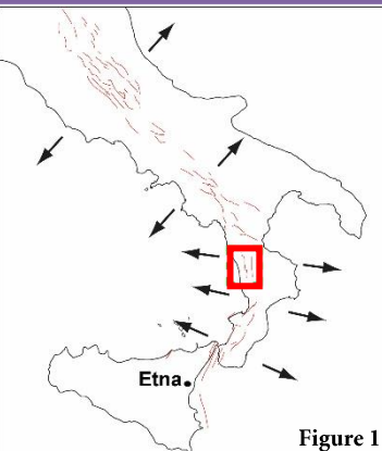
Active normal fault map of central and southern Italy with extension directions. (modified from Faure Walker et al. 2012)
