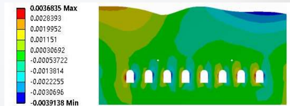
Y-direction distribution profile of displacement field without cracks
