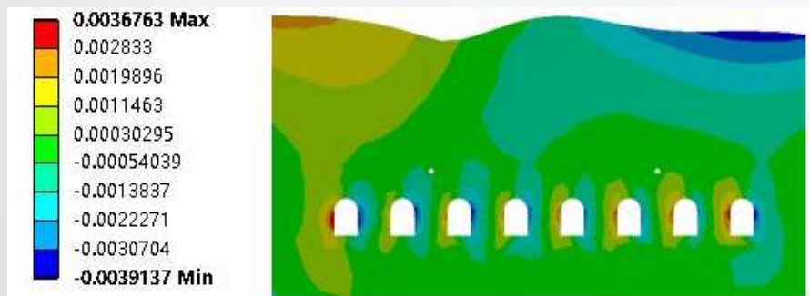
Y-direction distribution profile of displacement field with cracks
