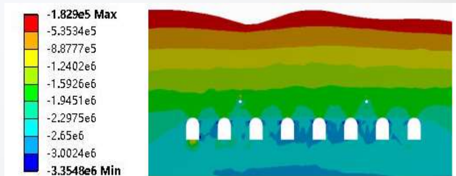
X-direction distribution profile of stress field without fracture
