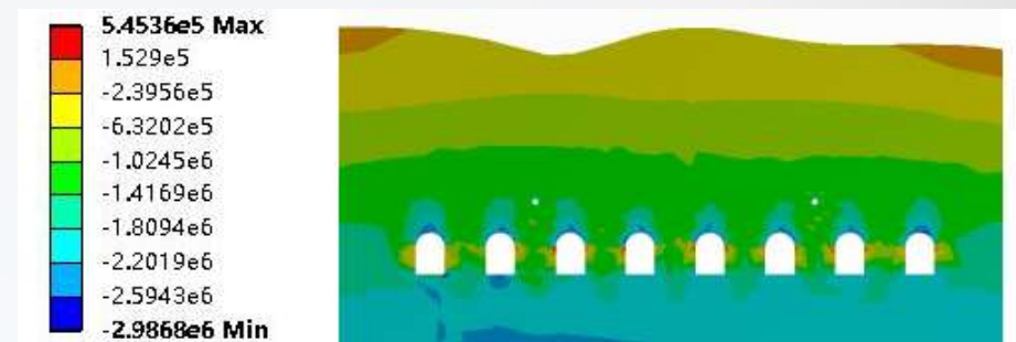
Y-direction distribution profile of stress field without fracture
