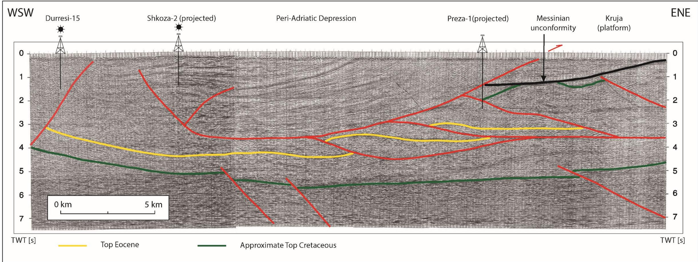
**Fig. 5.** Interpreted seismic (time) section across the outer Albanides (after Roure *et al.* 2004, modified; located in Fig. 2).
