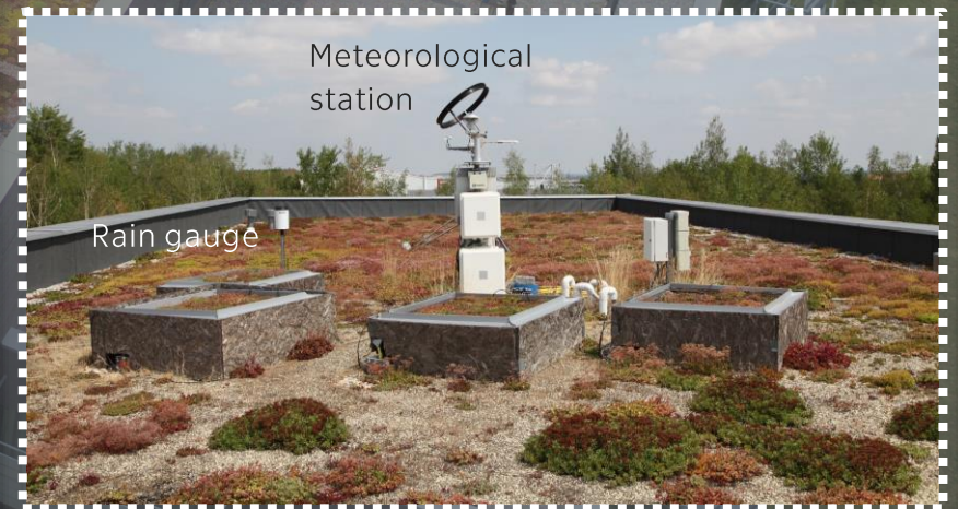
Fig. 1: Experimental site on the roof of the building with four green roof test beds.
